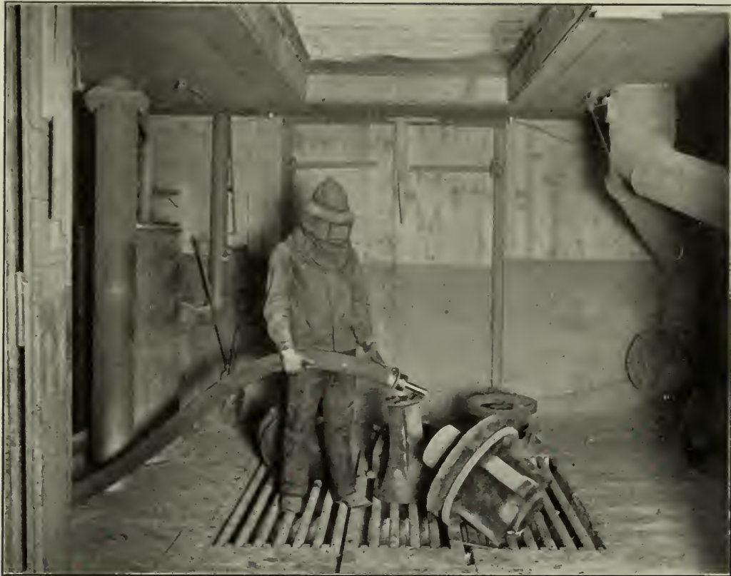
SAND-BLAST MAN READY TO PUT THE BLAST ON, SCHENECTADY SHOPS OF THE GENERAL ELECTRIC COMPANY.
